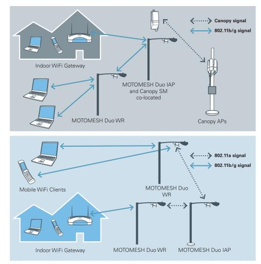
Figure 2: MOTOMESH Duo: Two Radio Solution There are benefits to each of the configurations, and decisions should be made based on user requirements. The two radio configuration can improve overall network throughput, reduce latency and enable more clients to be served by a single backhaul link.
